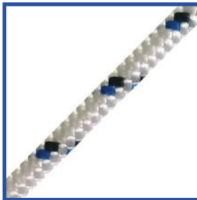
Q5170 3MM HMPE LEECH LINE BREAKING STRENGTH: 700KG CONSTRUCTION: POLYESTER SHEATH, HMPE CORE
